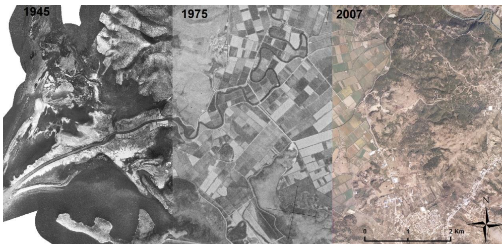
Figure 3. Series of aerial photographs (1945, 1975, 2007) used for the creation of thematic land use/land cover (LULC) maps and spatial matching following their geometric correction and adjustment. A section of Kalamas Delta is shown here as an example.
